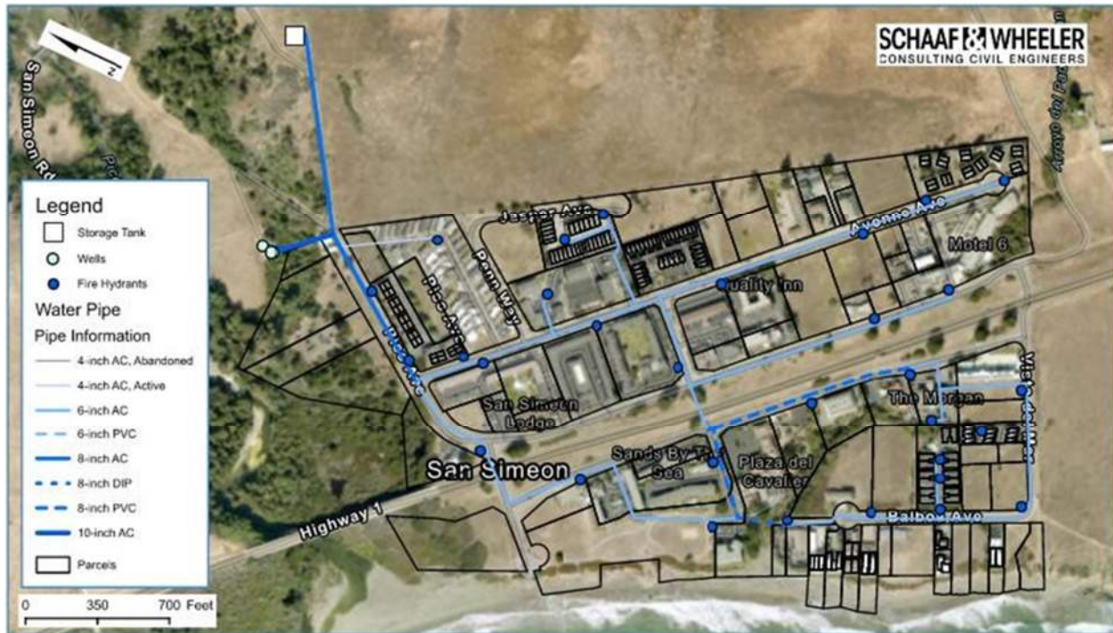
Figure 2. SSCSD Water System Overview
